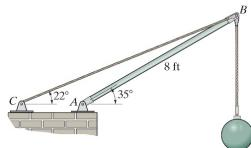
4. Determine the support reactions at fixed support A on the cantilevered beam.
