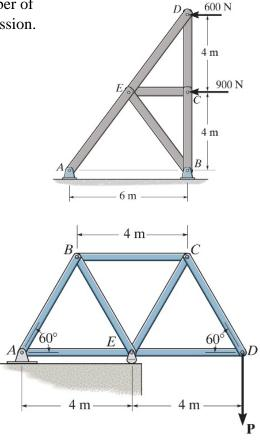
2. a) Use **method of joint** to determine the force in each member of the truss in terms of force P. Indicate the member is subjected to tension or compression. (hints: starting points from D, then C, B and E)
