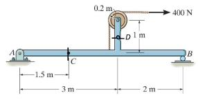
4. Draw the free-body diagram necessary to determine the internal force (N), shear force (V) and bending moment (Mb) on the cross section a) passing point D and b) passing point G. (G is 1 m above point B)
