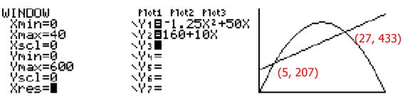
Use 5: intersect to find the values. State your window settings, sketch a graph (like above) and state: The company must produce 5,000 or 27,000 radios to break-even.
