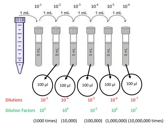
In this experiment we spread 100 uL samples from the last 5 tubes onto TSA plates. In order to determine the "effective dilution" on the surface of the plate, you have to multiply the dilution in the tube times the amount you put on the agar plate. We are using 100 uL. As you recall, 100 uL = 0.1 mL. We know that  $0.1 = 10^{-1}$ . Therefore, multiply the dilution for each tube by  $10^{-1}$ . The "effective dilution" on the surface of the agar plates is shown in red above.
