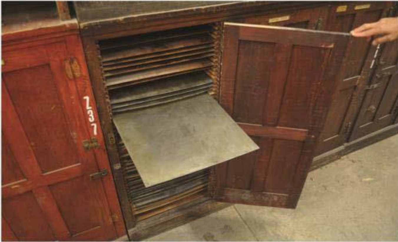
A ZINC PLATE IN ITS STORAGE CABINET. MOST PLATES WERE STORED HORIZONTALLY IN WOODEN CABINETS TO PREVENT TOUCHING AND WARPING (PHOTO COURTESY OF BRUCE GEYMAN, USGS)
