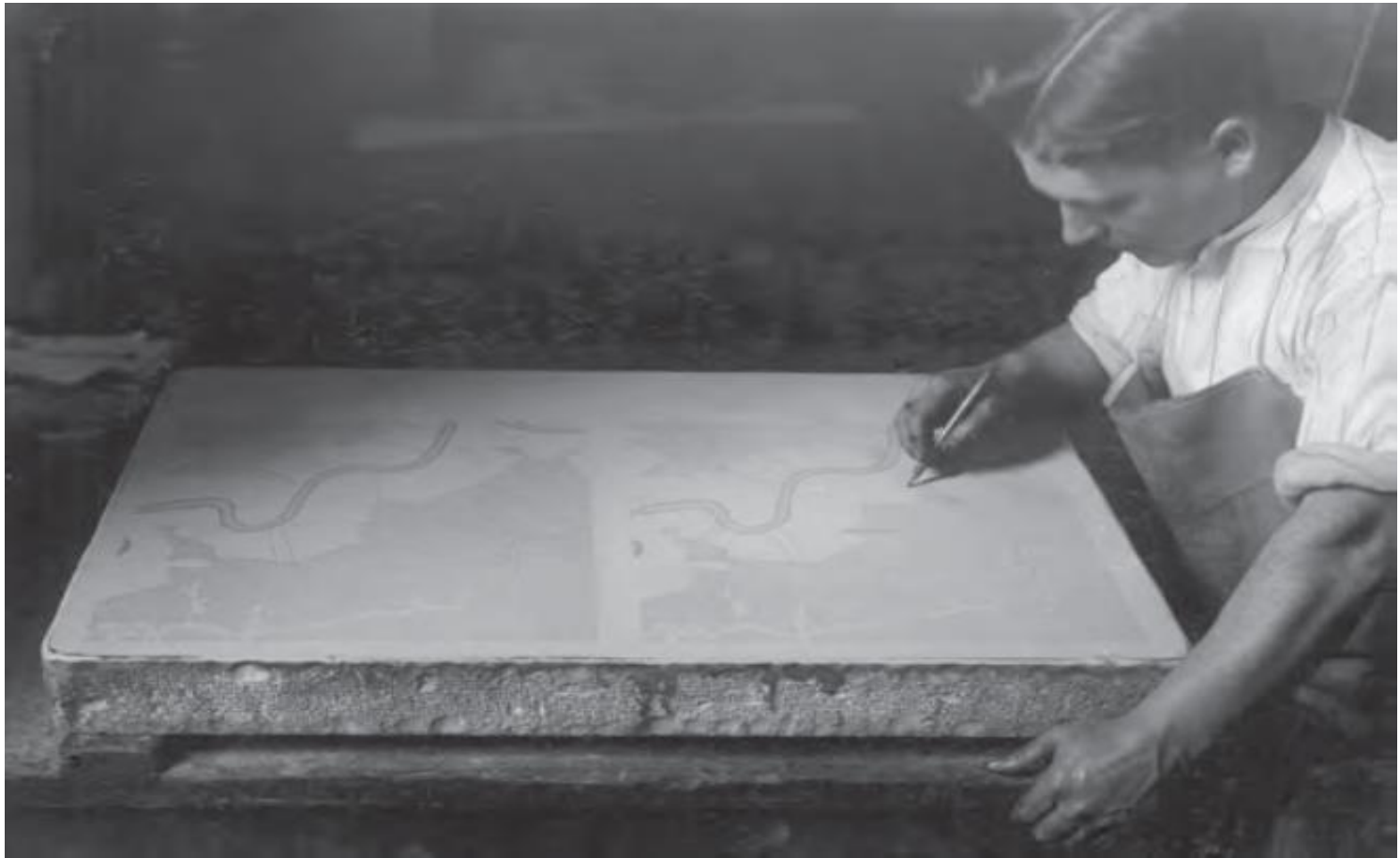
TOPOGRAPHIC INFORMATION WAS TRANSFERRED FROM COPPER OR ZINC PLATES TO A LITHOGRAPHIC STONE FOR PRINTING
