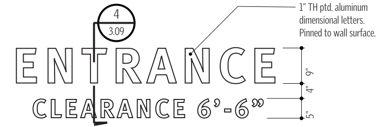
1 Elevation - Sign Type N1 1/2" = 1'-0"
