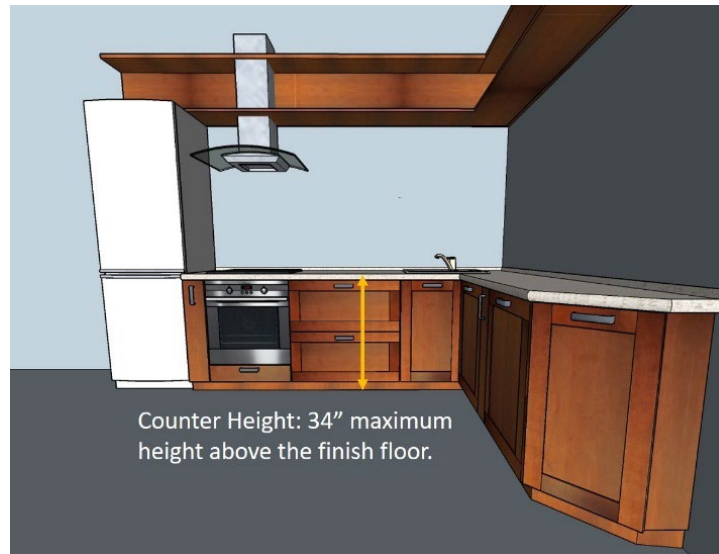
Figure 2-13 Accessible Dining and Work Surface
